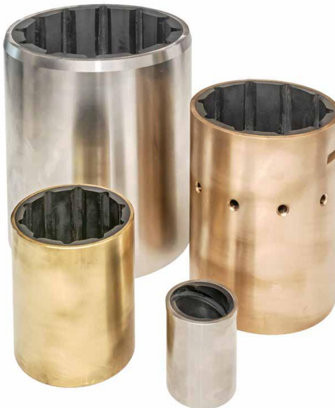
The flexibility of the bearing surface allows adjustment of the approach angle in response to an applied load to maintain water-wedges, acting in a similar manner to modern tilting pad thrust bearings to maintain the film thickness.
